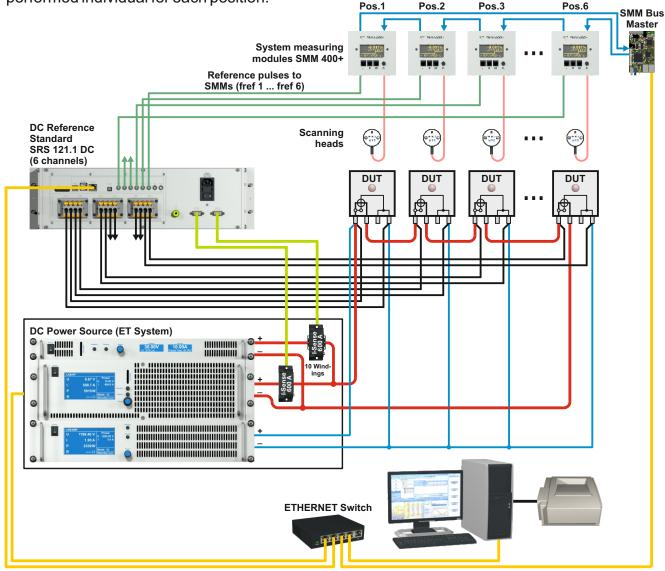
The DC Meter Calibration System is designed to test single-phase DC electricity meters with open and closed I-P links. It is fully electronic, using only solid state electronic components and is controlled by a PC via the integrated ethernet interfaces.
