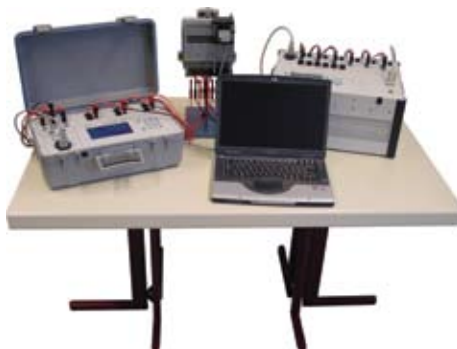
Single-position meter test set
